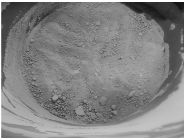
Fig. 7. Inside of the fluid bed dryer bowl mid-way through the vacuum transfer operation, showing both round balls and irregular lumps.
