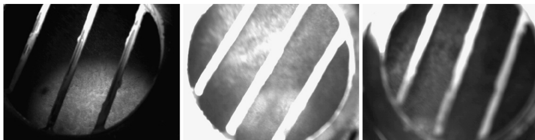
Fig. 5. View through the observation port of three different batches, showing visibly different powder flow and dust levels at identical impeller speed.
